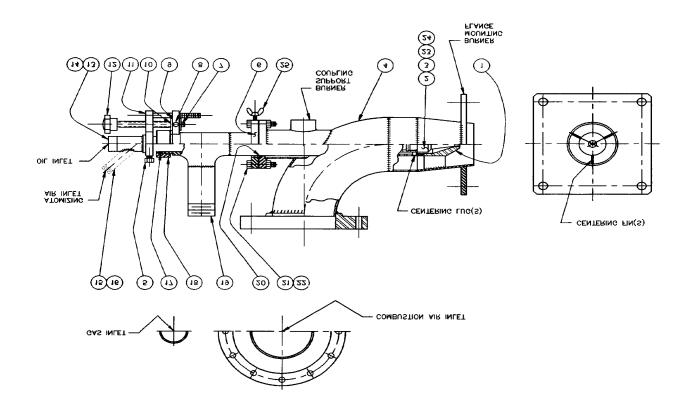
**Figure 3 - Hot Air Burner Parts Identification Drawing**
