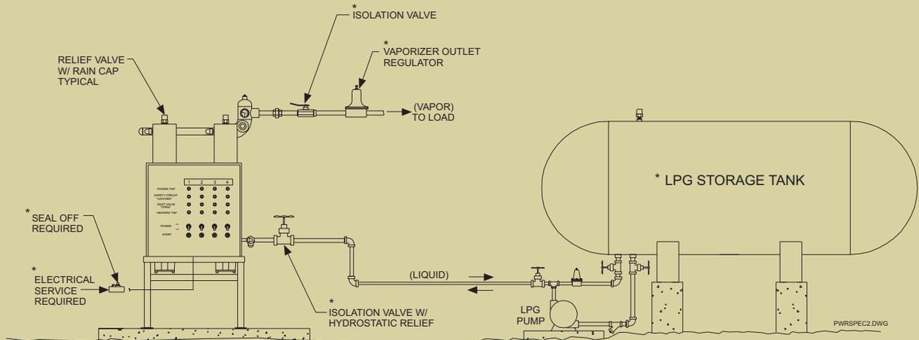
NOTE: NO CHECK VALVES IN LIQUID LINE; LIQUID MUST BE ABLE TO FLOW IN BOTH DIRECTIONS.
