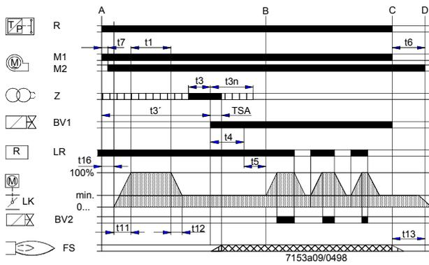
Modulating expanding flame burner
