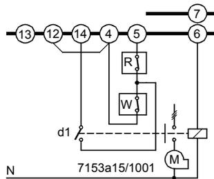
If an auxiliary contact «d1» of the fan contactor is included in the circuit as shown in the diagram, ignition and release of fuel take place only when the contact is closed.
