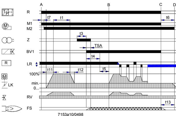
During burner off times, the air damper is fully closed.
