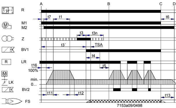
Control of actuator according to the single-wire control principle.
