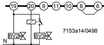
Relay is not required if «BV3» at terminal 20 is hydraulically series-connected with «BV2».
