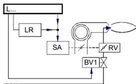
Load control with modulating controller with galvanically separated control contacts for positioning directions OPEN and CLOSE.
