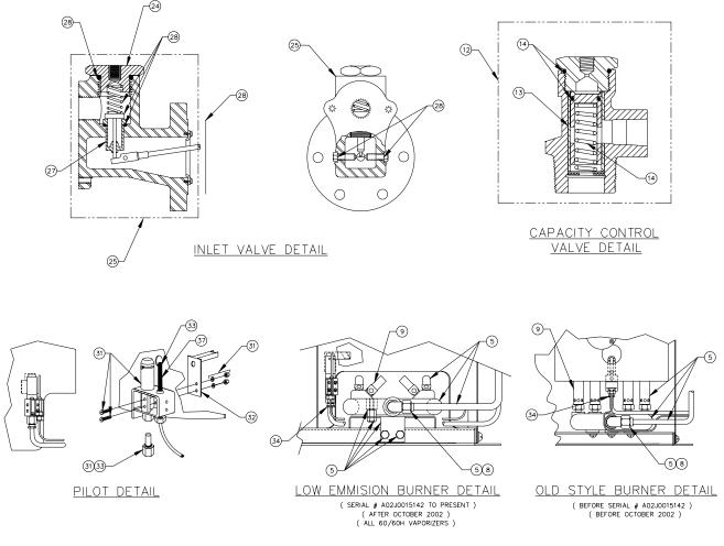
Figure 12 – 40/40H and 60/60H Vaporizers: Inlet Valve, Capacity Control Valve, Pilot and Burner Assemblies.
