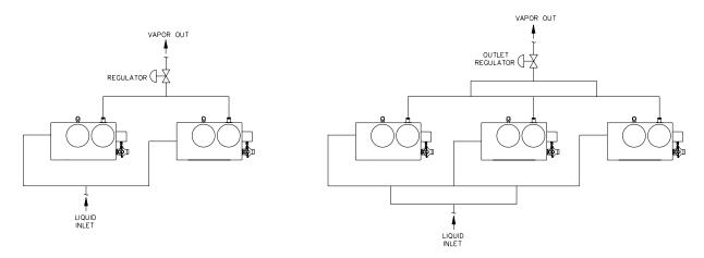
An oversized inlet and outlet manifold may be used to balance the flow.
