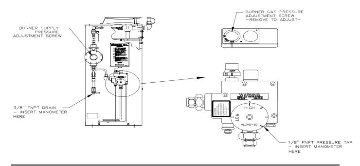
Figure 10 – Regulator and Thermostat Adjustment
