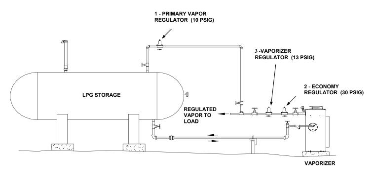
After installing the vaporizer, install and set the regulators from the economy kit as follows:
